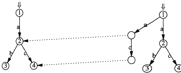
FIG. 2. Simply simulation equivalent, but not simply bisimilar, TSs
